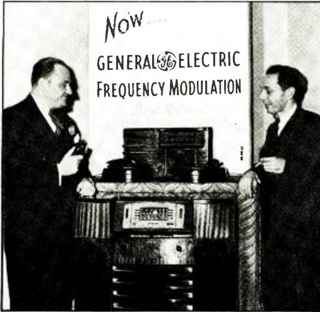
Demonstrator for G.E. F.M. sets, permits dealer to show how this transmission - reception operates free from man-made static, by playing record on wireless record player through F.M. and A.M. sets. Electric razor, well-known "static generator" is also feature of demonstration.
