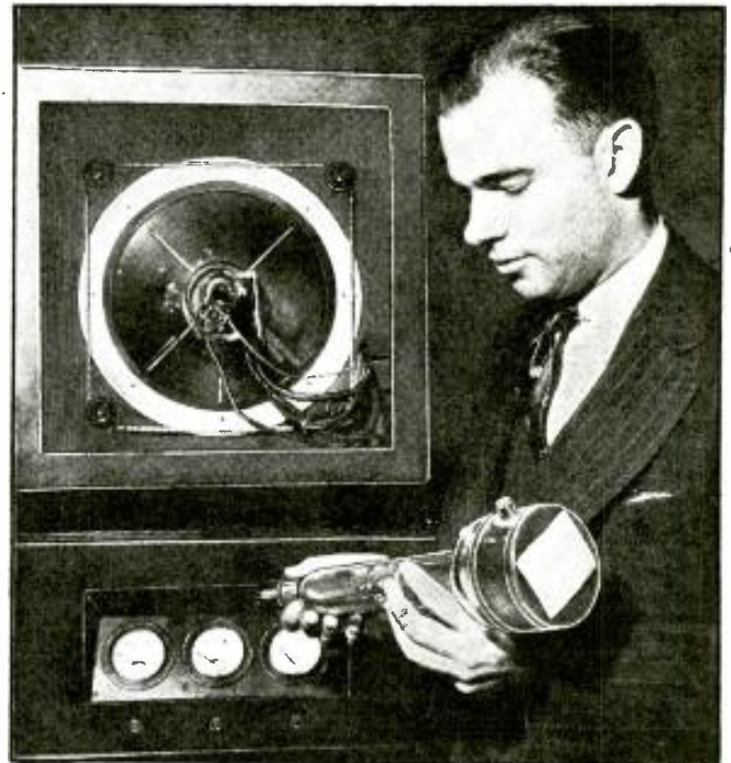
N.B.C.'s Ray Monfort, and projection Kinescope; left, projection lens.
