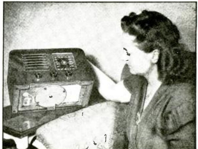
New "Roto Base" on RCA Little Nipper model 46X23 permits it to be turned in any direction, thus permitting the built-in loop antenna to be aimed directly at the wanted station thereby increasing signal strength.
