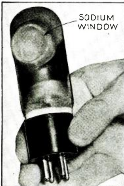
Window "bubble" passes U.-V. rays to sodium cathode.
